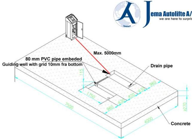
The hydraulic oil hose from the lift to the control box is 6000mm so it is recommended that the box is max. 5000mm from lift
