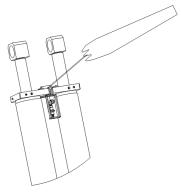
4. Screw loose the core of solenoid unloading valve fixed on the hydraulic block.
