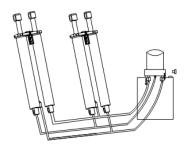
2. Connect the optional hand pump to the hydraulic block at the point where the removable plug used to be fitted.
