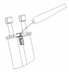
2. Screw loose the core of the solenoid unloading valve fixed on the hydraulic block.
