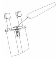
2. Loosen the core of the solenoid unloading valve fixed on the hydraulic block.
