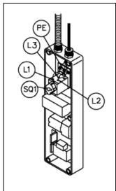
Before making any electrical connection please check the electrical supply voltage is the same than lift voltage mentioned in the lift specifications.
