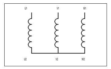
To connect 400V put the terminal-ends together U2-V2-W2 with a terminal stripand connect the mains from the Control box to the engine U1-V1-W1. Any intervention in the electrical circuit, even if it is not important, has to be made by the Official Technical Service of Jema Autolifte.
