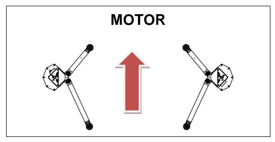
Before lifting the vehicle, check that the lifting arms are locked. When the car is in position, pushing the up button we will Lift the car until the button is released or until the upper limit switch is activated when maximum height is reached. Once
